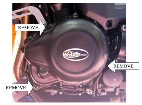
In this kit there should be: 1 x Engine Case Cover (ECC0136) 3 x M6x35mm long button head bolts
