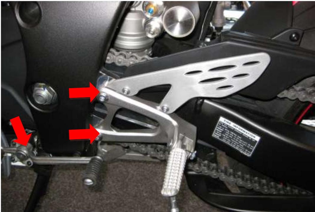
Remove the original rearset and shift-lever, but keep the original gearshaft and gearbox-connector.
