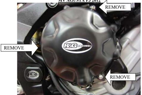
In this kit there should be: 1 x Engine Case Cover (ECC0147) 3 x M6x35mm long button head bolts
