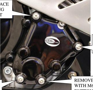
REMOVE AND REPLACE WITH M6x35mm LONG BUTTON HEAD BOLT
